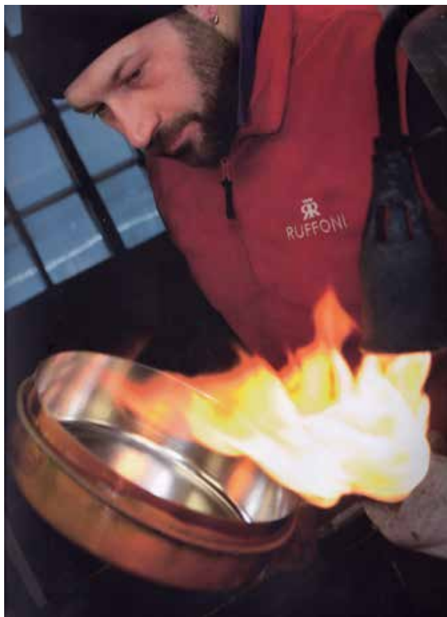
Alan "the fire-eater" skillfully hand tinning on the fire using high purity tin.
