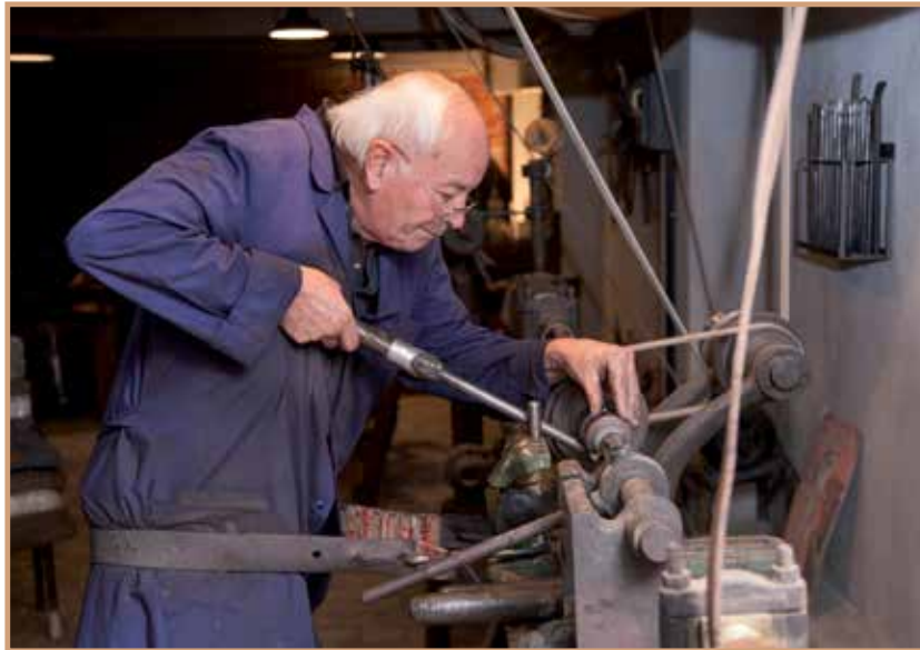
The hand copper-spinning. Franco making a cream caramel mold.
